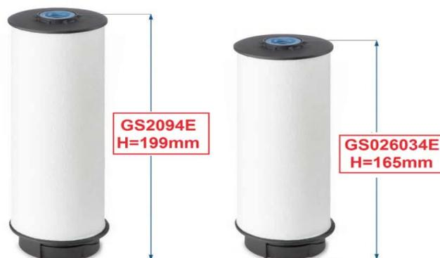
*The filter with code **TECNECO GS2094E** with applications on the new **IVECO DAILY EURO 6** engine has been developed with a particular filter media with high water-fuel separation, capable of retaining even the smallest water particles with dimensions not exceeding 5 microns.*
